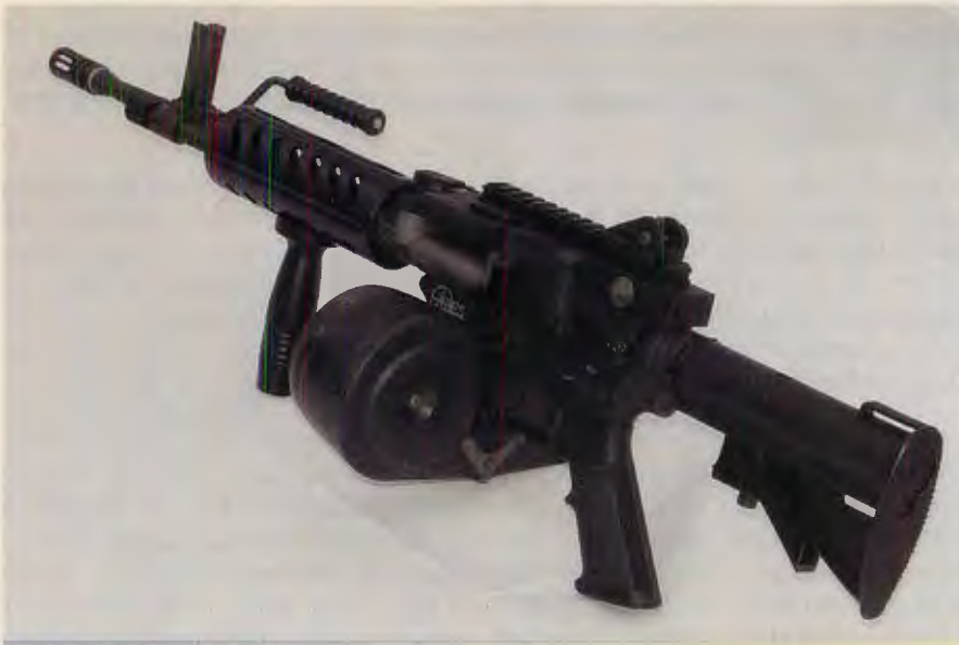
The Shrike 5.56-S (Standard) can fire either from a detachable magazine – box or drum as shown here with Beta Company 100-round C-MAG – or from a belt, depending on the mission.
